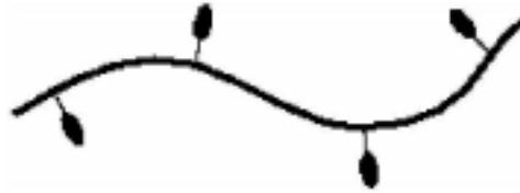
Fig. 10. Natural splines: metal stripes curved by "ducks".
