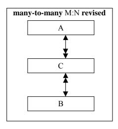
**Note:** In addition to the linking attributes, the (composite) table may also contain some relevant attributes. Also the creation of the linking table produces the desired 1:M relationships within the database. And especially note that the tables A and B now contain only one row for entity. Only the linking table contain redundancies.
