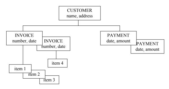
This occurrence of a hierarchical database record corresponds to the hierarchical structure (or model):
