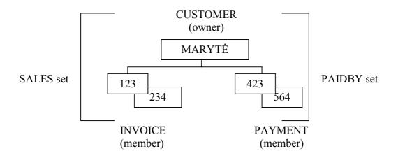
The DBMS automatically updates the pointers after the execution of each operation. A pointer exists for each record type in a set. A pointer's current value refers to a **current record**. Actually, two types of currency pointers exist:
