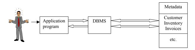
10 pav. The DBMS Manages the Interaction Between the End User and the Database.
